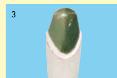
The varnishes are translucent. If they are applied several times, the colour becomes more intense so that the layer thickness can be controlled.
