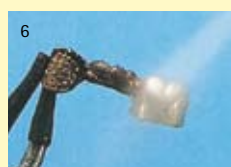
Always apply a fresh coat of Oxyd-Stop-PM after the casting has been heated. Only then is optimum protection against oxidation provided.
