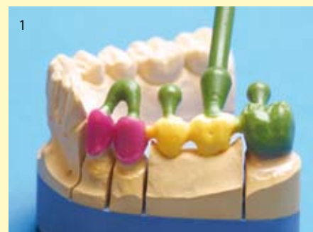
The double rinsing heads are used for two objects with the same volume. Attaching is easier and the amount of work is reduced.
