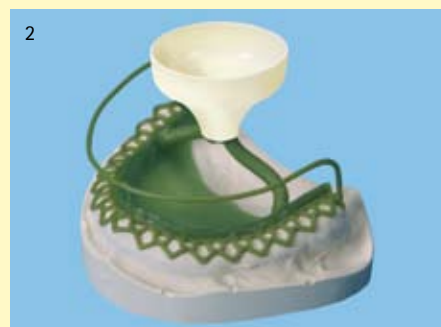
During casting the compressed air is displaced into the air channels and produces castings free from shrinkage cavities, which can be easily fitted.
