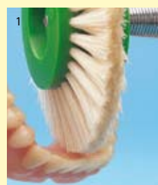
The wet, mixed pumice diffuses into the brush and nonwoven fibre fabric (Abraso-Soft Acrylic).
