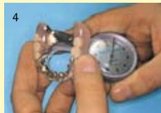
The dial caliper is used to measure the thickness of the outer telescopes.
