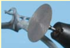
Separating and grinding back the sprues.
