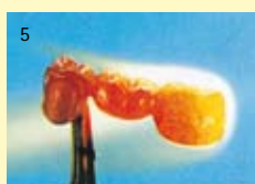
Always apply a fresh coat of Oxyd-Stop-PM after the casting has been heated. Only then is optimum protection against oxidation provided.
