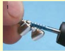
Precious metal technique: Smooth surface of the object, tool is running steadily.
