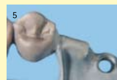
Preheat the investment model slightly (50-100°C). Super-flux will fill the soldering gap more easily. Apply only a small quantity of Superflux.
