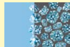
Diamond crystals embedded in a special mixture of binding material.
