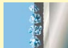
Diamond crystals in an electro-deposited metal bond.
