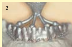
Even very small tensions in the low-cost and biocompatible single-piece casting process are perfectly compensated.
