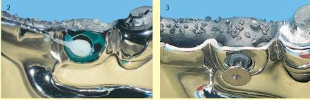
Sandblast metal parts with 110µm aluminium oxide (pressure: 3-4 bar). Use FGP separating agent tioned lock. for areas that are not bondedd. Wet with MKZ Primer or use Silano-Pen.
