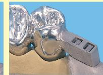
Conditioned double-T adhesive connector ready for bonding with DTK-adhesive.
