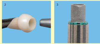
The adhesive titanium base is fixed in the model analog. FGP separating agent - a varnish which provides protection and serves as an indicator when the polished rim is accidentally damaged during sandblasting - is applied to the rim (transition towards the implant interface).
